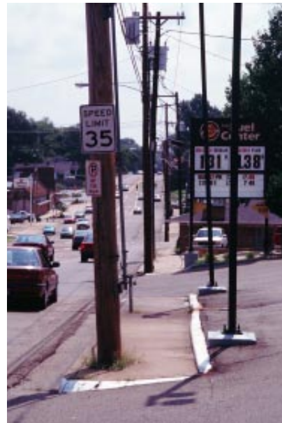
Narrow sidewalks with many poles as obstacles need to be redesigned and repaved to create better pedestrian paths.
